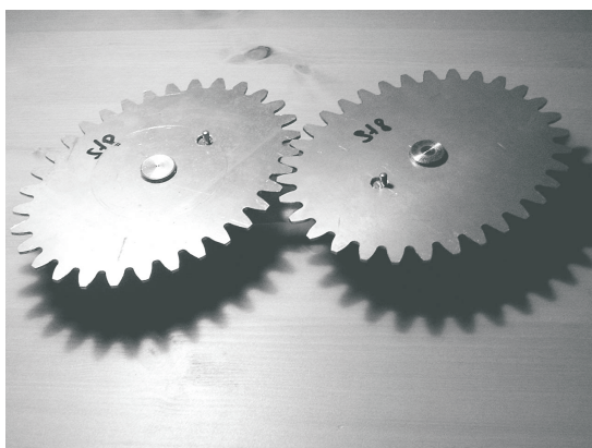
Fig. 13. Non-circular gear on checking fixture
